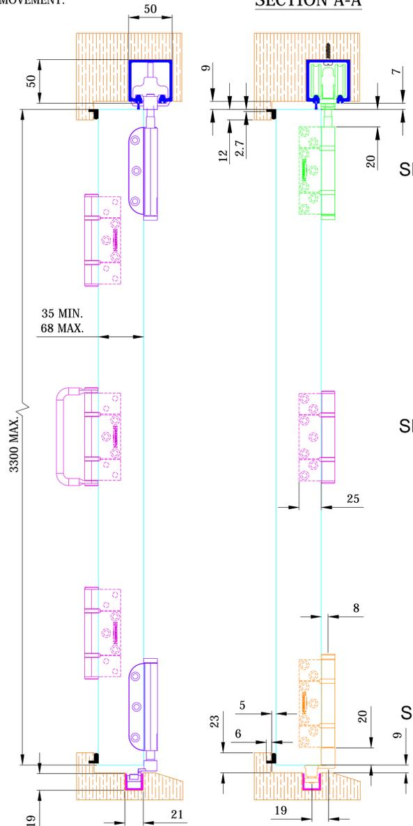
WHEN USED IN CONJUNCTION WITH THE ALUMINIUM SUPPORT CHANNEL
